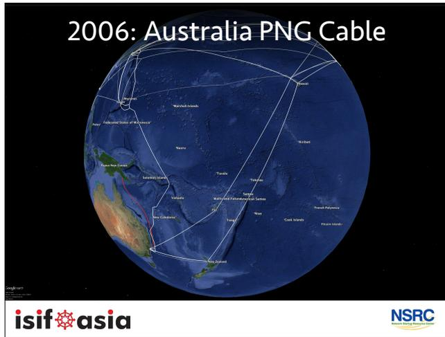
2006 has the cold, dead snake of PacRim West dragged off the seafloor and hauled to Port Moresby - recommissioned with a design bandwidth of just over a gigabit per second. From what I understand, regeneration in this cable is electronic, not optical, and E5 (565mbps) is as fast as electronic regeneration will work. So we've got two 565mbps pairs bringing a total of 1.1 gigabit per second into PNG.
