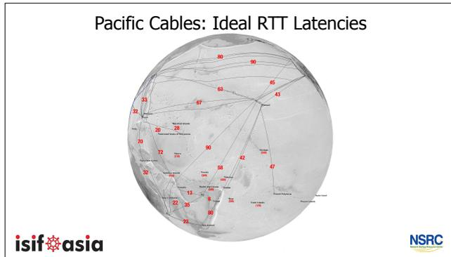
So let's go back to all that new cable infrastructure. Talking to cable operators & measuring cable segment lengths I've constructed a simple model of network latencies to look at how all these cables should be performing. Numbers are RTT in milliseconds. It all looks great. It's hard to find any combination of paths that would reach the quarter-second threshold for human perception.
