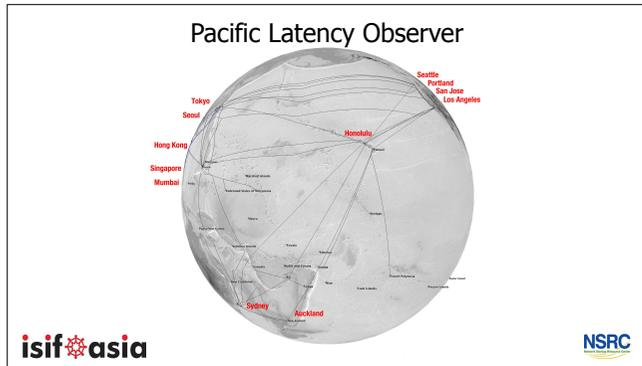
Theory is all well and good, but to test out these assumptions, I've set up servers around the world measuring latency into Pacific networks every five minutes. There they are, dotted around and on the globe.
