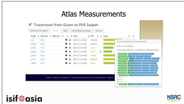
Some of the types of measurements I'm doing with Atlas are traceroutes. Here I've run a test from seven hosts in Guam on three different carriers to another carrier on Saipan, in the Northern Marianas.
